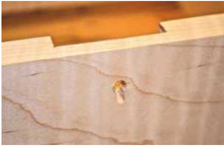
▲ Pic.10 After determining which side would be the front, I started cutting out for the half mortise lock and key hole
